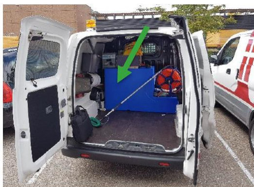
Figure 1: A look inside one of AFA JCDecaux' e-NV200 electric service vans. The grey box on the top of the blue water tank holds the LPS unit.
